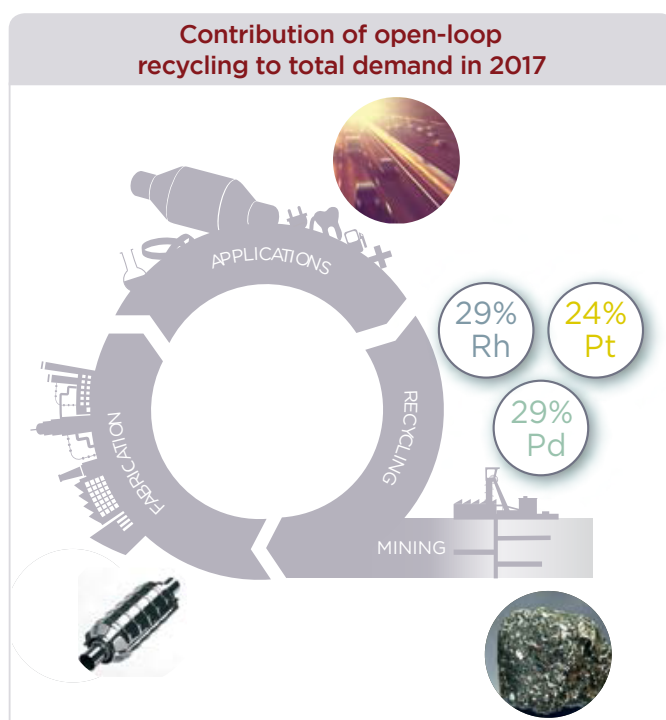
Figure 9: Life cycle of PGMs; image credit platinum ore: Johnson Matthey; recycling numbers based on Johnson Matthey PGM Market Report, May 2018.
