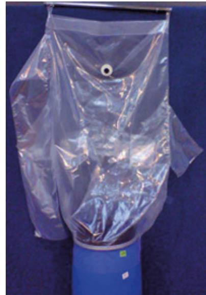
Figure 9-5(b): Glovebags used in vacuum transfer of material from dryer bowl and for sampling containment
