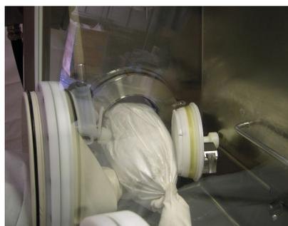
Figure 9-21(b): Alpha door opened to allow passage of material
