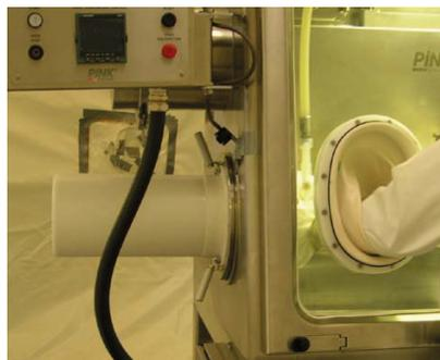
Figure 9-21(a): Beta canister docked to isolator
