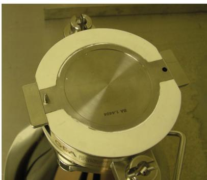
Figure 9-18: The passive half of a split butterfly valve attached to a container
