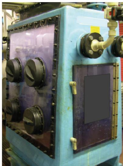
Figure 9-3: Glovebox with gloveport shields
