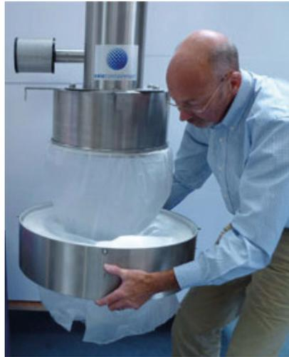
Figure 9-16: Cassette preloaded with liner
