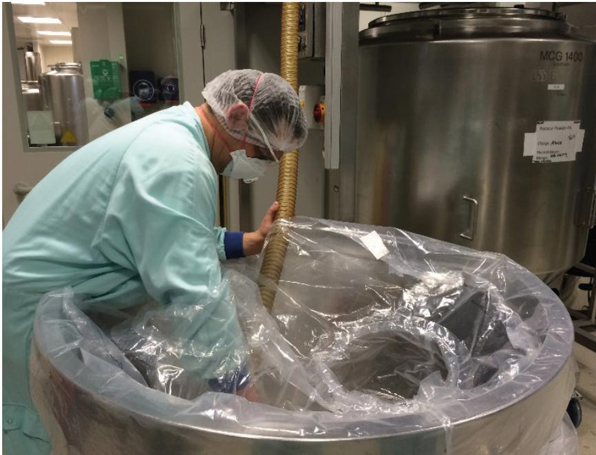
Figure 9-5(a): Glovebags used in vacuum transfer of material from dryer bowl and for sampling containment (courtesy of Solo Containment)
