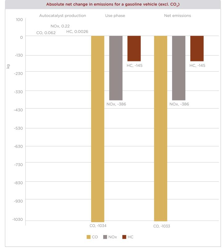
Figure 6: Absolute net change in emissions for a gasoline vehicle (excl.  $CO_2$ ).
