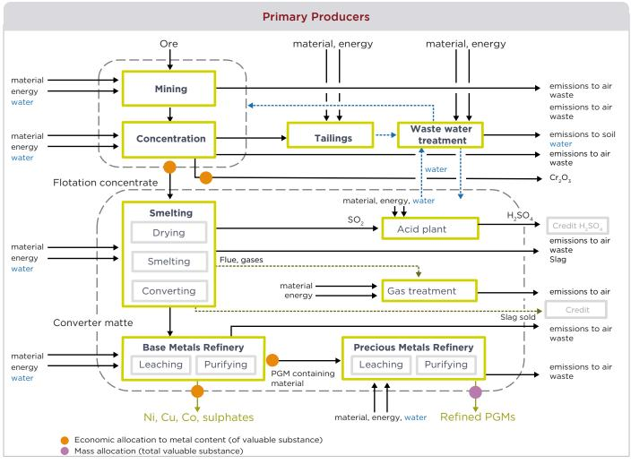
Figure 3: Allocation for the primary production route
