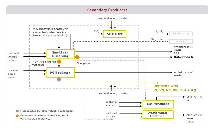
Figure 4: Allocation for the secondary production route
